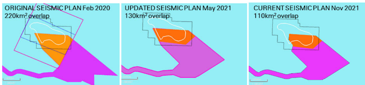
Figure 7: Comparing the change in overlap for planned seismic acquisition: (Left) original Seismic acquisition plan using traditional three dimensional (3D) towed streamer; (Centre) new plan using 3D high resolution seismic with shorter streamers, prior to RLB change in Hornsea 4's DCO application; (Right) new plan using 3D high resolution (HR) with shorter streamers, after the RLB change in Hornsea 4's DCO application.
